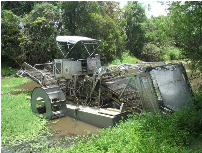
6: The weed harvester used to mechanically remove the weeds and open the creek channel.
