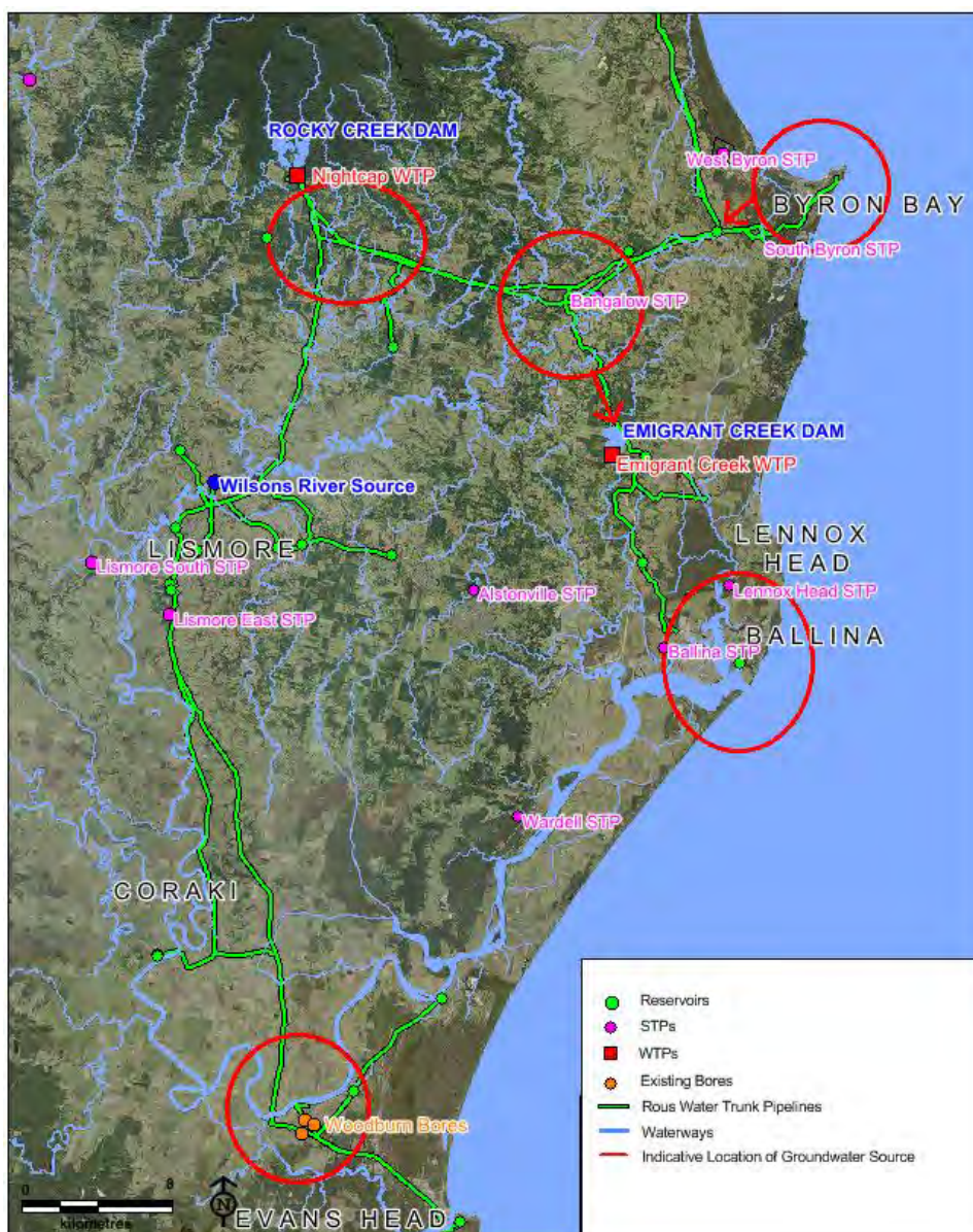
Figure 6-5: Scenario 3 – prospective location of groundwater sources
