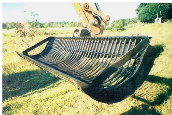
Reed buckets are the preferred excavation equipment when removing weeds from waterways.
