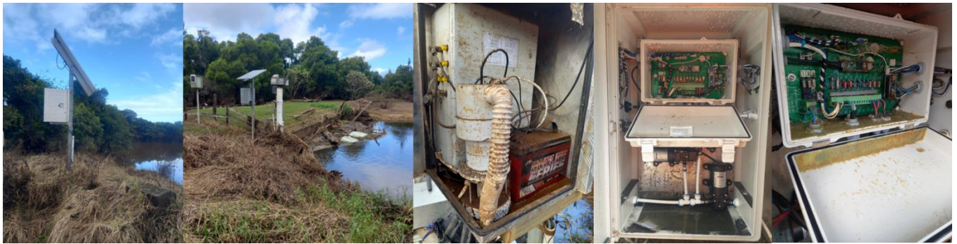
Figure 3 Photos of flood damaged loggers
