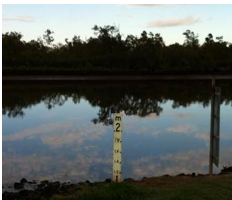
Figure 4-5 Depth marker style gauge used for water level (Emigrant Creek boat ramp)
