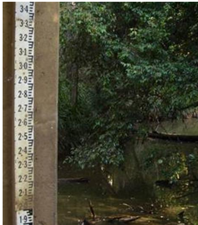
Figure 4-2 Flat gauge plates with 0.01m markings (Rappville)
