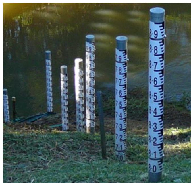
Figure 4-3 Half-round gauge plates with 0.01m markings (Eltham)
