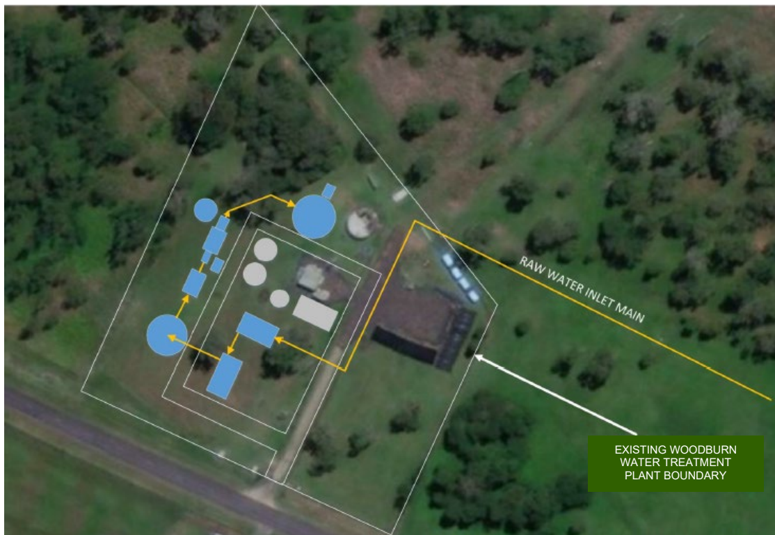
Figure 14: Woodburn groundwater WTP inlet and layout
